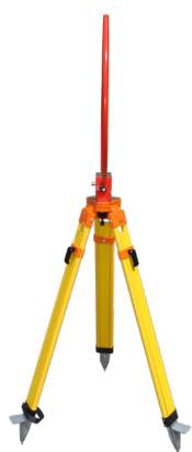
HLA 6121, mounted on tripod CTP 6099, Y position
